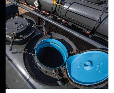
Series 391 Tank Armor is built to resist high concentrations of chemicals that can wreak havoc on transport vehicles.
