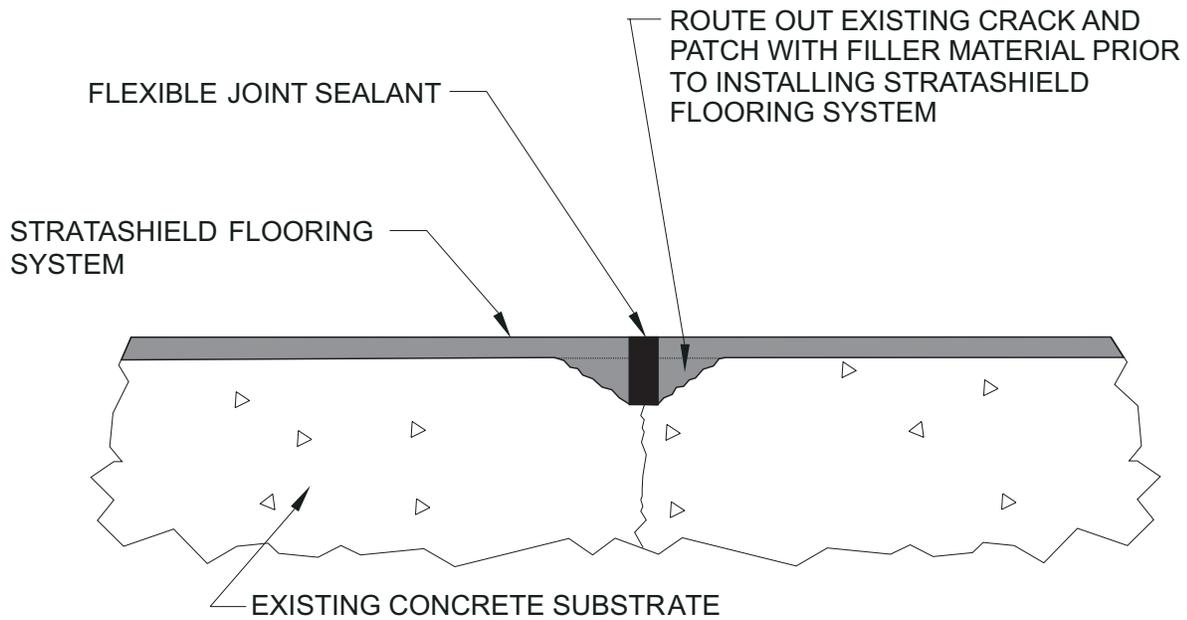
NOTE: USE SERIES 215 OR STRATASHIELD 100% SOLIDS EPOXY MIX WITH FUMED SILICA, SILICA FLOUR OR FINE AGGREGATE FOR FILLER MATERIAL
