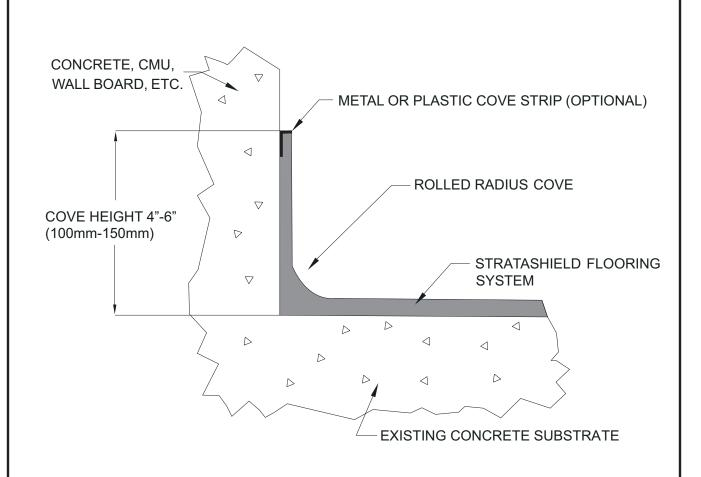
NOTE: USE DRY MIXED TROWELABLE MORTAR VERSION OF FLOORING MATERIAL TO BUILD COVE.
