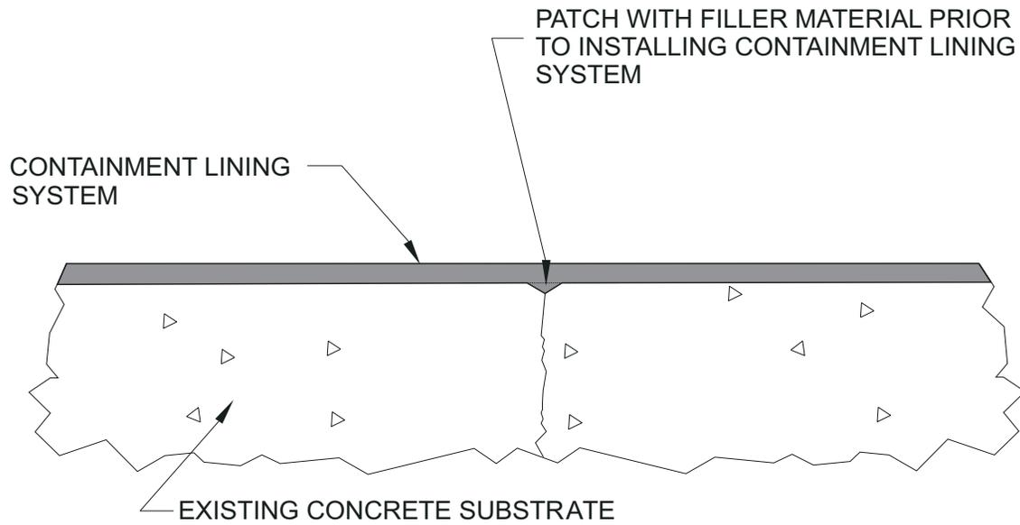
NOTE: USE SERIES 215 OR SERIES 201, 237SC, OR 239SC 100% SOLIDS EPOXY MIXED WITH FUMED SILICA OR SILICA FLOUR FOR FILLER MATERIAL. ROUTE OUT CRACK PRIOR TO PATCHING IF CRACK IS LARGER THAN 1/16" (1.58mm).
