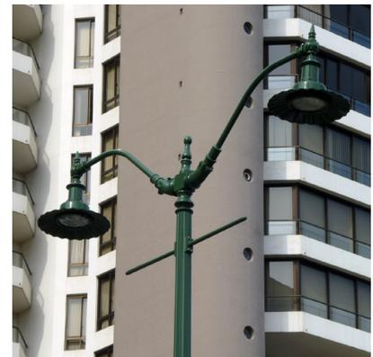
Tnemec Series 1070 Fluoronar protects the antique-style lampposts in Waikiki, Hawaii, from UV light, as well as damaging coastal conditions.
