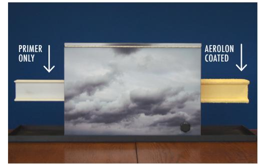
Here, an I-beam runs through a container filled with ice, replicating a cold exterior environment. The left side, which is unprotected, serves as a control. The right side is coated with Aerolon at 100 mils.
