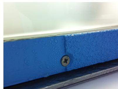
Condensation can be limited by applying the Aerolon coatings system to window frames. This display shows the difference in condensation between one side (right) sprayed with Aerolon and the other (left) uncoated.
